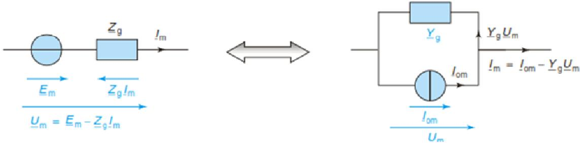
$$\underline{U}_m = \underline{E}_m - \underline{Z}_g \underline{I}_m \Rightarrow \underline{I}_m = \frac{\underline{E}_m}{\underline{Z}_g} - \frac{\underline{U}_m}{\underline{Z}_g} \quad \frac{\underline{E}_m}{\underline{Z}_g} - \frac{\underline{U}_m}{\underline{Z}_g} = \underline{I}_{om} - \underline{Y}_g \underline{U}_m$$
