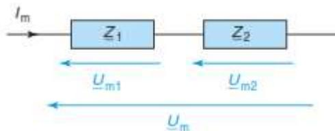
$$\underline{U}_{1m} = \frac{\underline{Z}_1}{\underline{Z}_1 + \underline{Z}_2} \underline{U}_m$$
