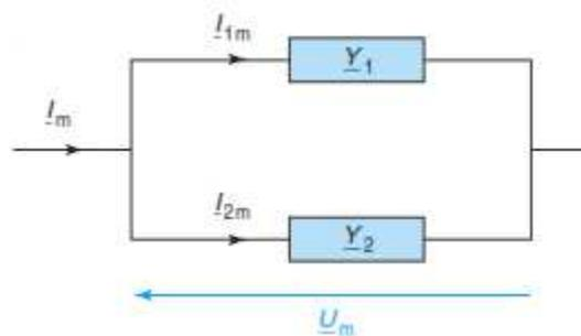
$$\underline{I}_{1m} = \frac{\underline{Z}_2}{\underline{Z}_1 + \underline{Z}_2} \underline{I}_m = \frac{\underline{Y}_1}{\underline{Y}_1 + \underline{Y}_2} \underline{I}_m$$
