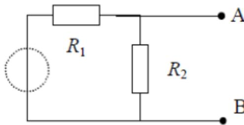
$$r = R_{eq} = \frac{R_1 R_2}{R_1 + R_2}$$
