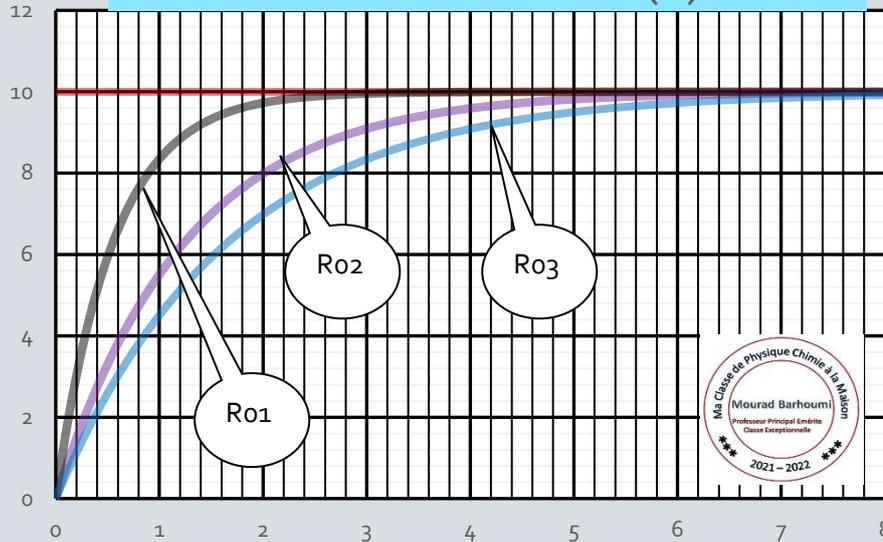
$R_{01} = 180 \Omega$  ;  $R_{02} = 80 \Omega$  ;  $R_{03} = 60 \Omega$
