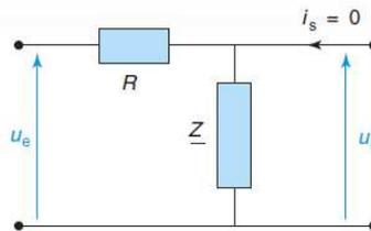
$$\underline{H}(j\omega) = \frac{u_s}{u_e} = \frac{\underline{Z}}{R_1 + \underline{Z}} = \frac{1}{1 + R_1 \underline{Y}}$$
