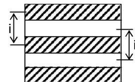
$$\text{Pour les franges brillantes, } i = x_{K+1} - x_K = (K + 1) \frac{\lambda D}{a} - K \frac{\lambda D}{a} \Rightarrow i = \frac{\lambda D}{a} ;$$
