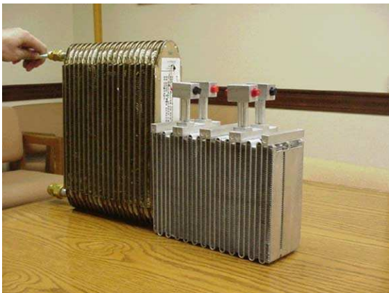
Fig. 39. Conventional (left) and prototype (right) CO 2 evaporator for mobile air-conditioner.
