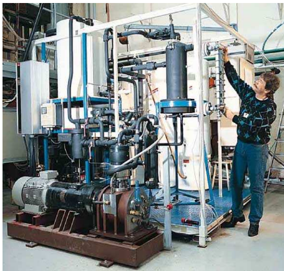
Fig. 55. Fifty kilowatt prototype heat pump water heater in SINTEF/NTNU laboratory [108].
