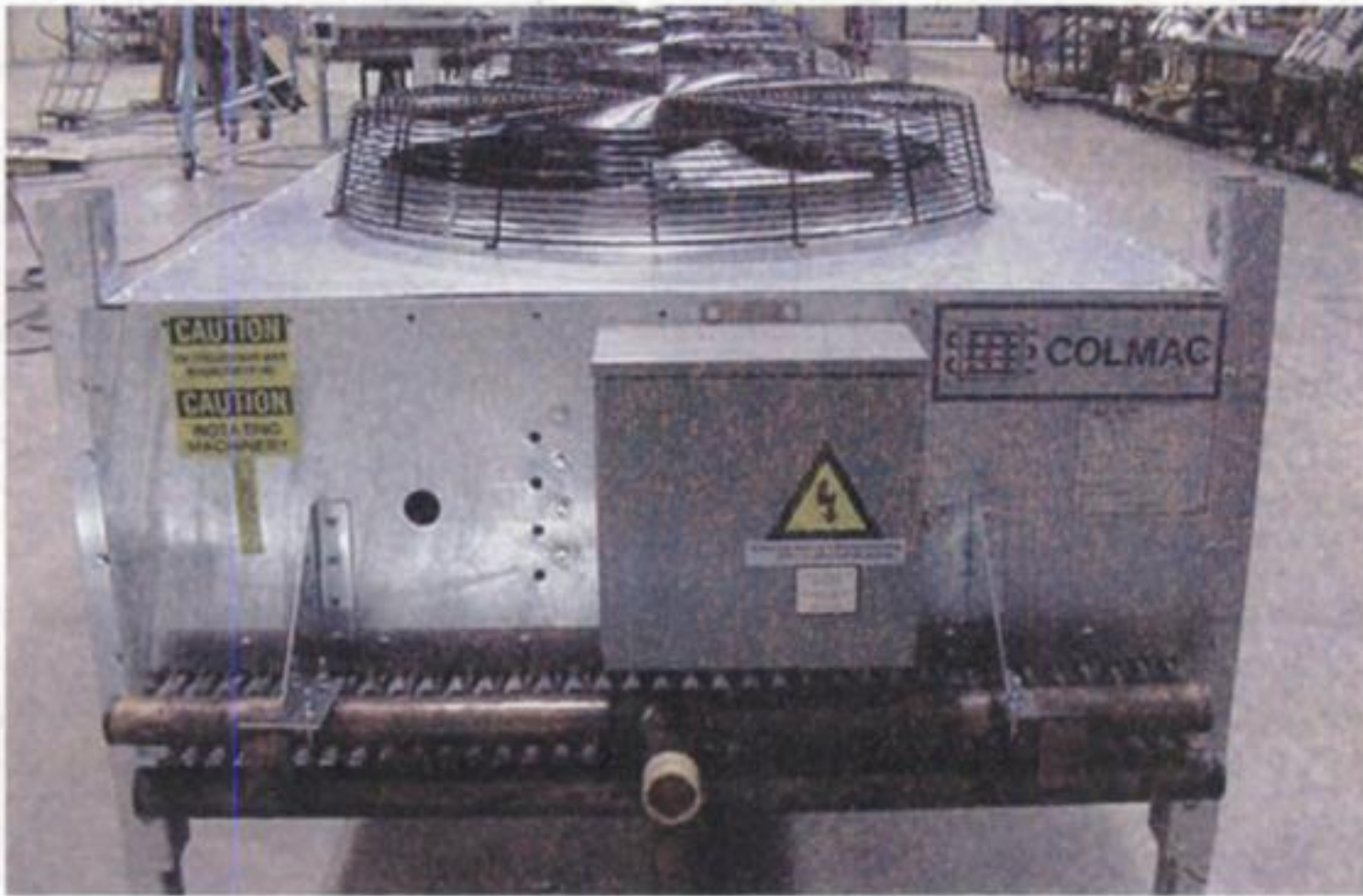
Air cooled condenser.
