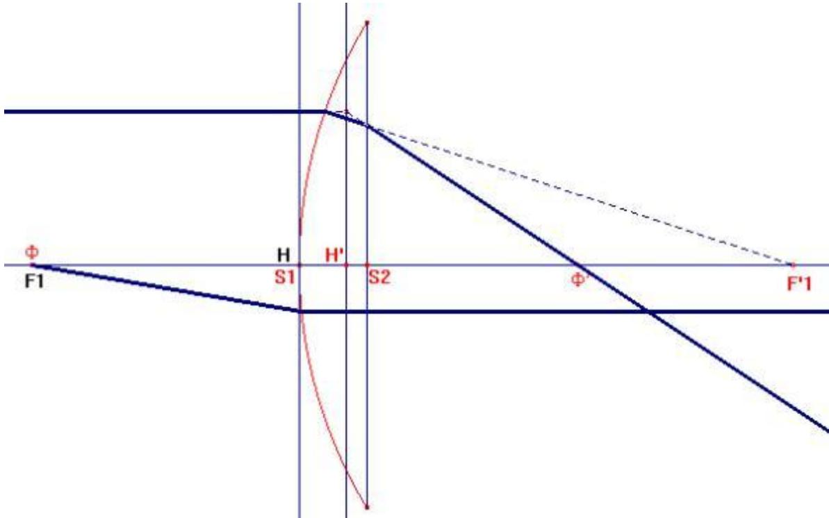
$$\overline{H\Phi} = \overline{S_1\Phi} = -\frac{\overline{S_1C_1}}{n-1}$$
